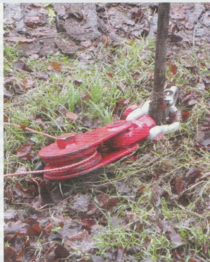
Mike Gardner showing how to use a cant hook, with logs laid out on beams to make moving easier (above). He positioned a snatch block (left) on a bar with string just to show the safe way to position winches and cables when pulling logs. He favours a snatch block with removable cheeks so that a rope or cable can be inserted more easily. Mike also added that signs are important in a woodland as visitors may appear on a footpath (below)
