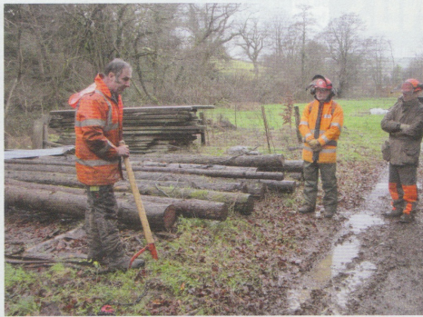
Mike Gardner showing how to use a cant hook, with logs laid out on beams to make moving easier (above). He positioned a snatch block (left) on a bar with string just to show the safe way to position winches and cables when pulling logs. He favours a snatch block with removable cheeks so that a rope or cable can be inserted more easily. Mike also added that signs are important in a woodland as visitors may appear on a footpath (below)
