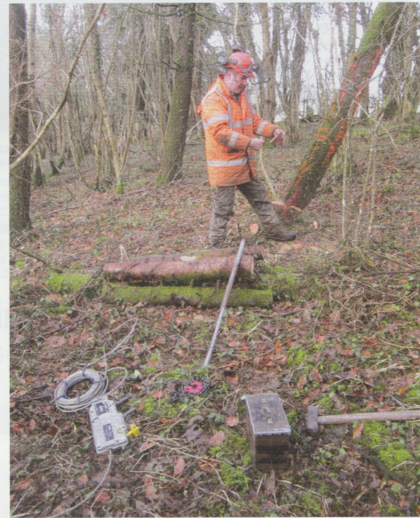
A small Tifor winch (above) about to be used for pulling back the bottom of a hung-up tree. Mike carries various wedges (below), but the steel ones can damage a chainsaw
