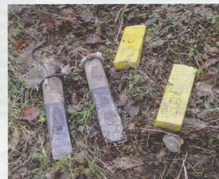
A small Tifor winch (above) about to be used for pulling back the bottom of a hung-up tree. Mike carries various wedges (below), but the steel ones can damage a chainsaw
